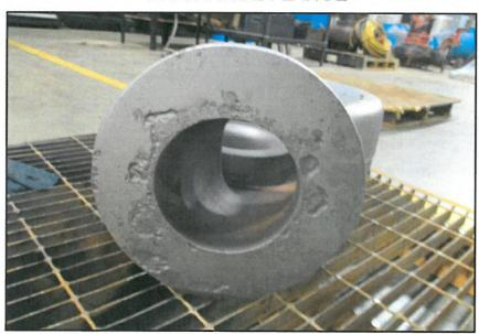
Ceramic coat volute discharge flange to restore surface conditions and help reduce future wear.
