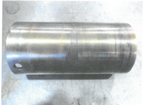
Corroded sleeve area on left and shaft sleeve on right
