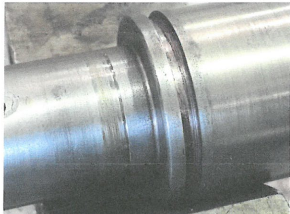
Shaft on left, lip seal fretting on right
