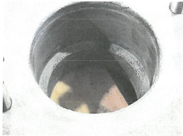
Stuffing box on left with corroded gasket area on right
