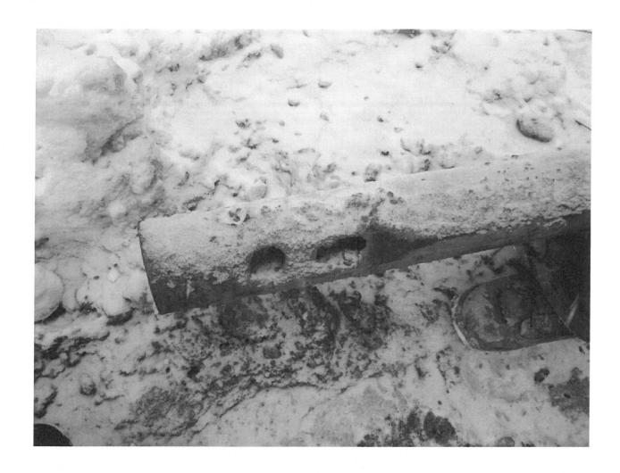
A section of the 1936 watermain removed in the railroad right-of-way. The holes punched through by the foreman just stepping on the pipe.
